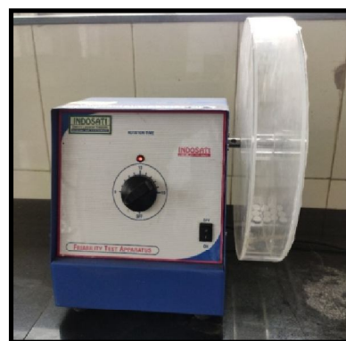
Fig No. 4 : Determination of Friability using INDOSAT Friabilator
